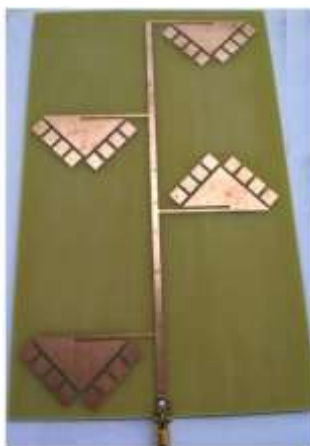
Fig.12. Fabricated Proposed 4x1 EBG Patch Array
